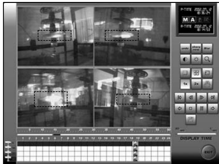
Fig. 3 Typical snap shots of the insulator flashover on the insulator surface.
